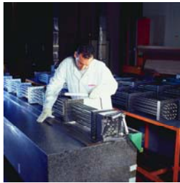
Fabricating fuel for pressurized water reactors (PWR) at the FBFC plant in Romans (France).
