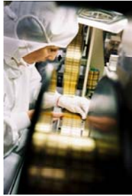
Manufacturing connectors for smart cards. FCI plant at Mantes-la-Jolie (France).
