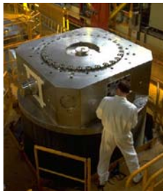
Maintaining and servicing shipping casks. COGEMA-La Hague plant (France).
